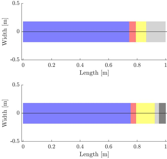
**FIGURE 7:** Plot of uniform beam, with optimal joint separation. Shaded regions indicate distinct rigid links.
