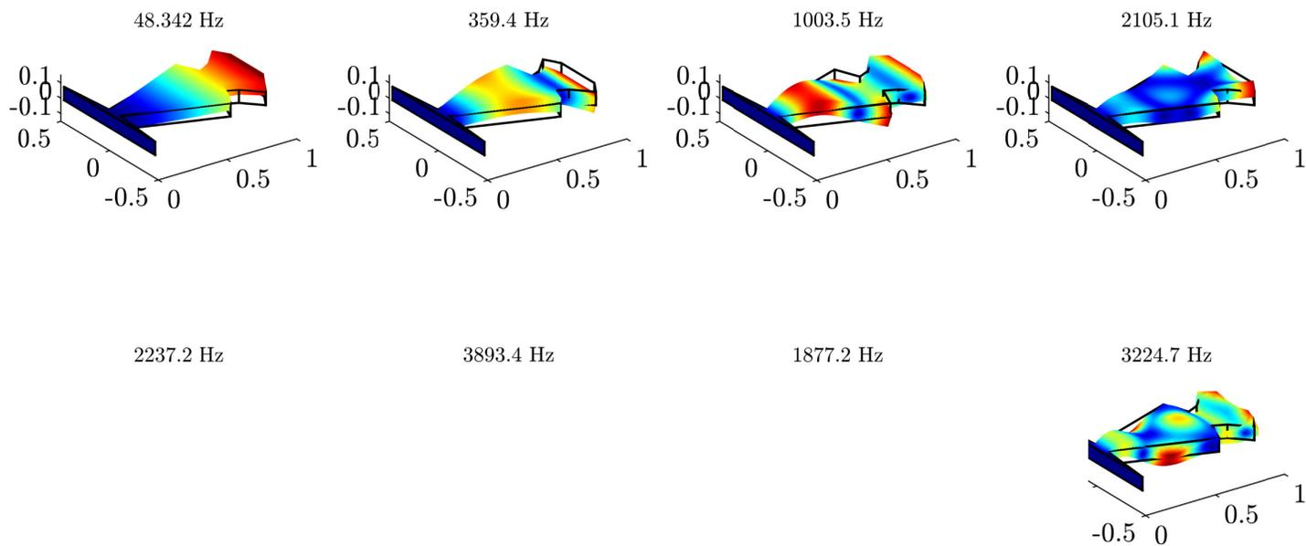
**FIGURE 13:** Plot of bending modes for 16 filtered eigenvalues, the title for each plot shows the resonant frequency, all axis lengths are in meters
