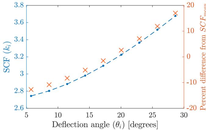
**FIGURE 8:** Plot of the spring Stiffness Correction Factor (SCF) vs. deflection angle (in degrees), for the 4R-PRBDM uniform beam. The right-hand axis corresponds to the relative change from mean values (Eqn. 24).
