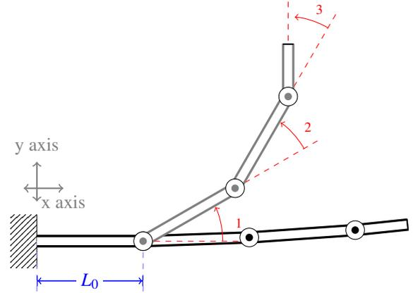
**FIGURE 3:** A 3R PRBDM at 2 different poses, the grey pose is the position when  $\theta = + \times \text{ones}(1,3)$ , and the black pose is for  $\theta = - \times \text{ones}(1,3)$
