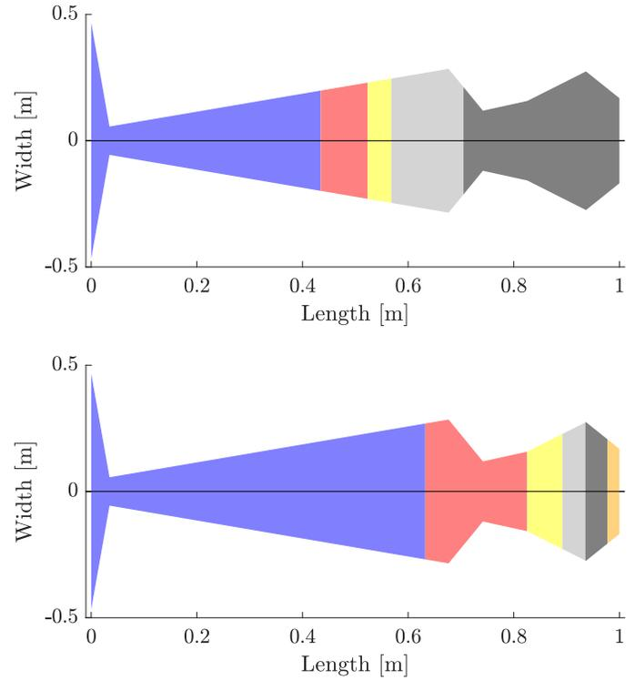
**FIGURE 11:** Plot of randomly general beam, with physical properties for each optimal section (5R-PRBDM)
