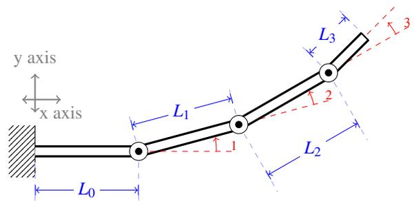
FIGURE 1: Illustration of 4-link/3R PRBDM
