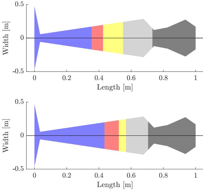
**FIGURE 9:** Plot of randomly general beam, with physical properties for each section optimized for eigenvalue matching (4R-PRBDM)
