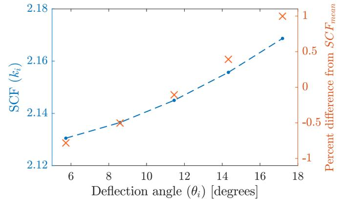
**FIGURE 12:** Plot of Spring Stiffness Correction Factor (SCF) vs. deflection angle (in degrees), for the 5R-PRBDM random beam case
