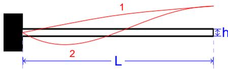
FIGURE 5: Side-view of a uniform beam of length  $L$ , thickness  $h$ , and width  $b$ . The red curves show the first 2 bending modes of the cantilever beam
