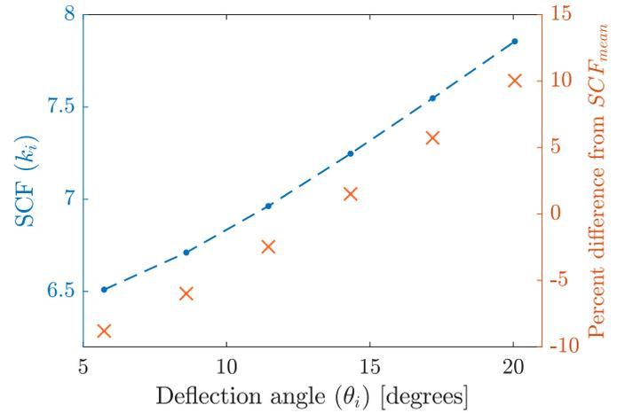
**FIGURE 10:** Plot of the spring Stiffness Correction Factor (SCF) vs. deflection angle (in degrees), for the 4R-PRBDM random beam case. The right-hand axis corresponds to the relative change from mean values (Eqn. 24).
