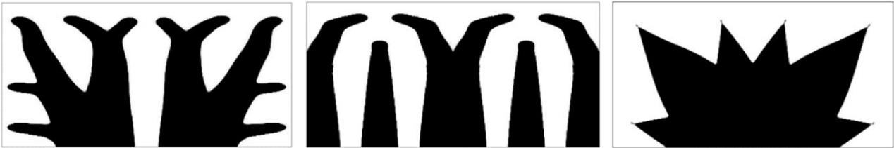
Figure 4. SIMP topology optimization solutions for thermal compliance objective. Pure conduction (left), conduction with uniform convection (center), conduction with boundary-dependent convection (right).
