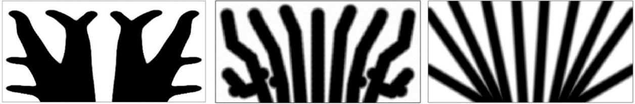
Figure 3. Topology optimization solutions for thermal compliance. SIMP method (left), space-colonization algorithm (center), geometric projection method (right).
