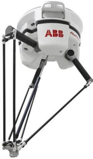
FIGURE 6: The ABB Flexpicker<sup>®</sup>
