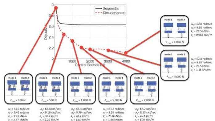
Figure 1. Transition from passive to fully-active suspension system design, and analysis of optimal designs throughout this transition.
