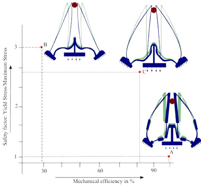
Figure 8. Designs obtained by maximizing the distributed compliance metric (C) maximally overcome the trade-off between minimizing stresses (B) and maximizing mechanical efficiency (A)
