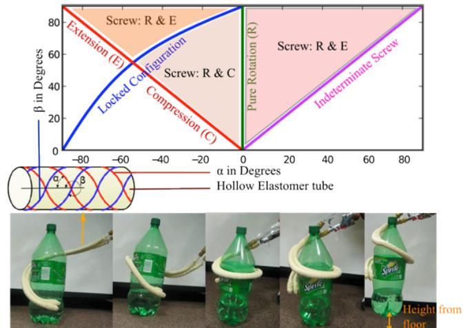
Figure 9. Using the wide unexplored design space for fiber-reinforced elastomeric enclosures to realize dexterous, adaptable manipulation
