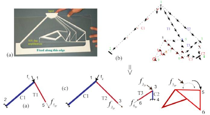
Figure 7. Subdividing a complex compliant mechanism topology into building blocks by assessing the nature of load flow. Members with axial load flow are transmitters(T) and transverse loads are constraints (C). A building block consists of one transmitter and one constraint.
