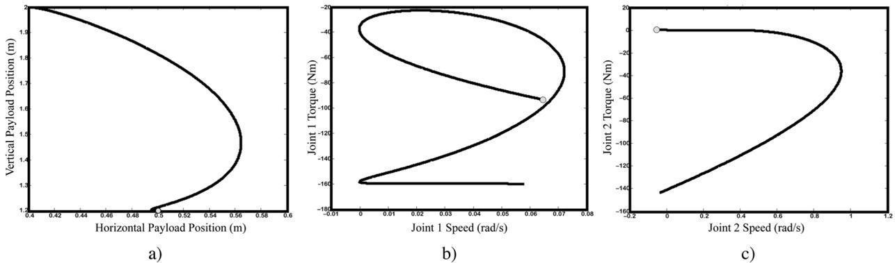
Fig. 6 Task B limited redesign results ( $\min E(x)$ ): (a) Payload trajectory, (b) joint 1, and (c) joint 2 torque-speed trajectories
