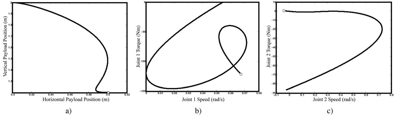
Fig. 4 Task B co-design results: (a) Payload trajectory, (b) joint 1, and (c) joint 2 torque-speed trajectories
