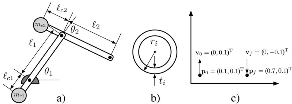
**Fig. 1 (a) Counterbalanced two-link planar manipulator, (b) section view of link  $i$ , and (c) task A initial and final conditions**
