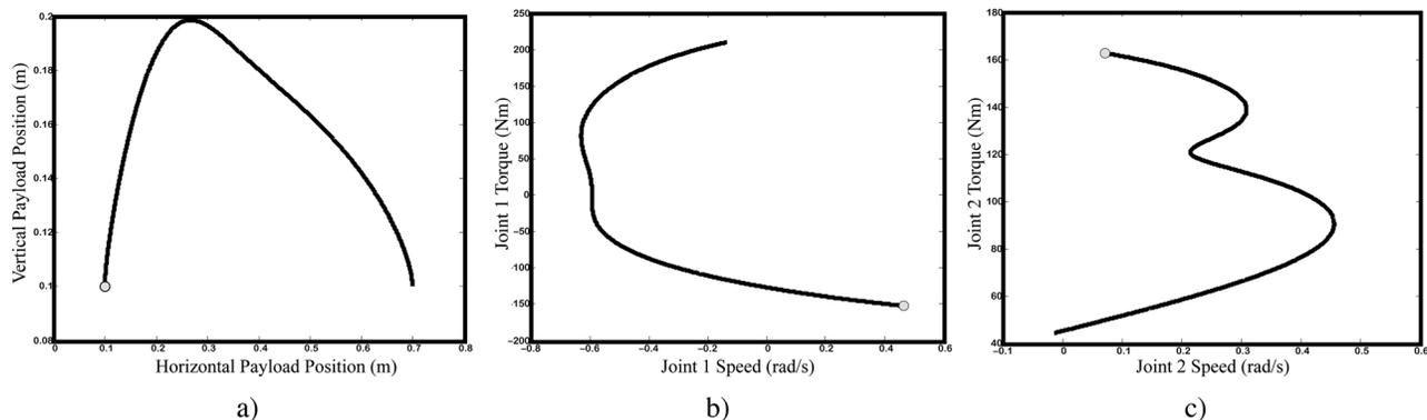
Fig. 2 Optimal trajectories for nominal plant design: (a) Payload trajectory, (b) joint 1, and (c) joint 2 torque-speed trajectories
