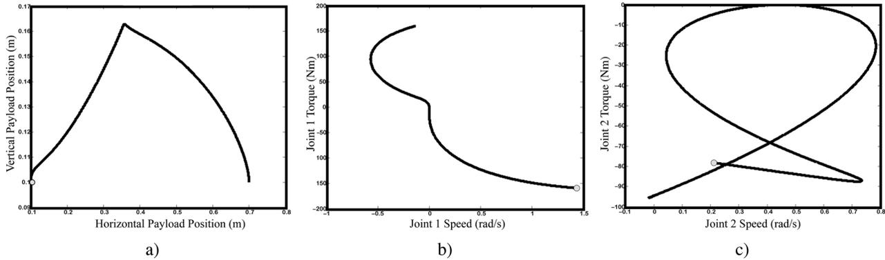
Fig. 3 Task A co-design results: (a) Payload trajectory, (b) joint 1, and (c) joint 2 torque-speed trajectories
