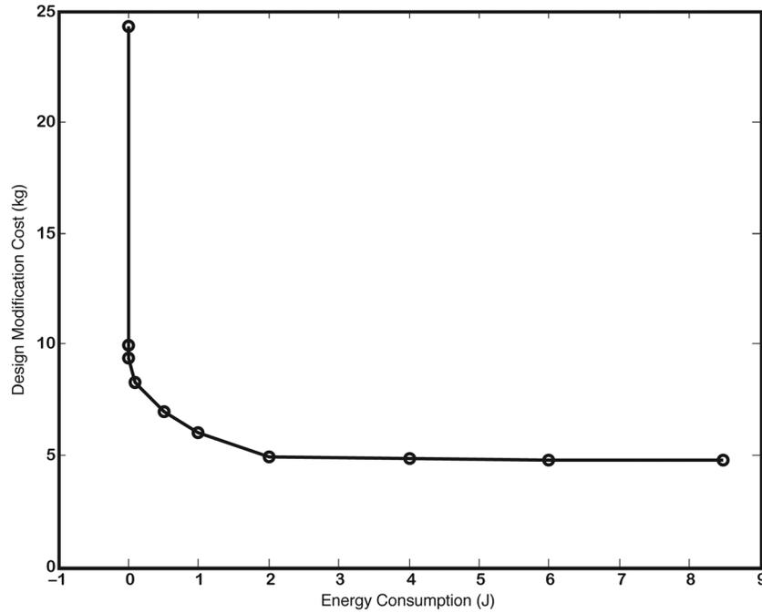
Fig. 5 Pareto set illustrating the tradeoff between energy consumption and plant redesign cost
