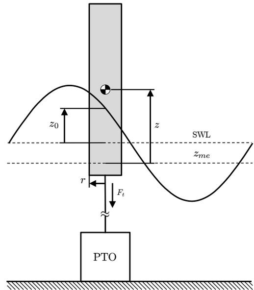
Figure 1: Tethered heaving cylinder wave energy converter.
