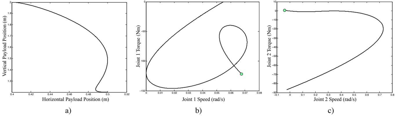
Figure 4: Task B co-design results: a) Payload trajectory b) Joint 1 and c) Joint 2 torque-speed trajectories.
