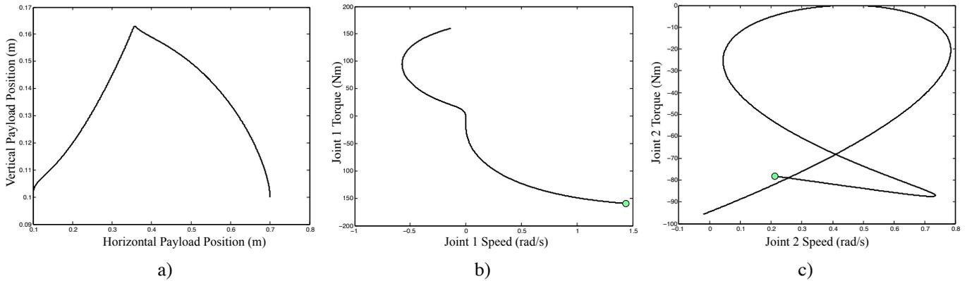
Figure 3: Task A co-design results: a) Payload trajectory b) Joint 1 and c) Joint 2 torque-speed trajectories.
