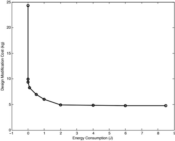
Figure 5: Pareto set illustrating the tradeoff between energy consumption and plant redesign cost.
