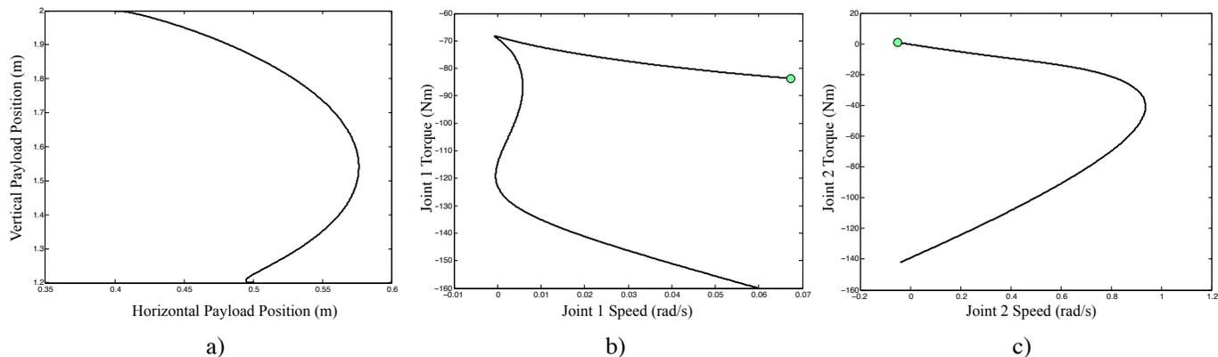
Figure 7: Task B PLCD results ( $E \leq 0.001$  J): a) Payload trajectory b) Joint 1 and c) Joint 2 torque-speed trajectories.
