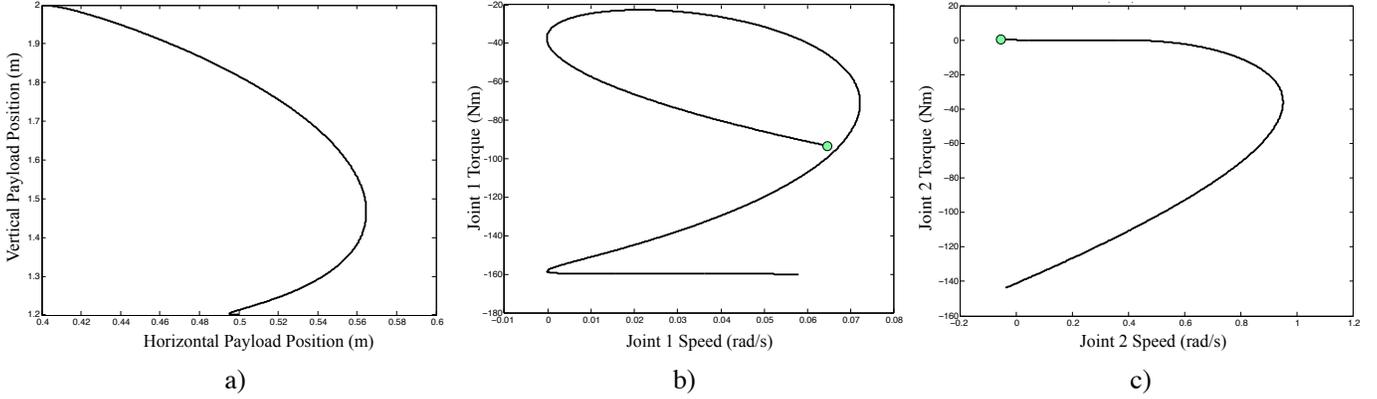
Figure 6: Task B limited redesign results (min  $E$ ): a) Payload trajectory b) Joint 1 and c) Joint 2 torque-speed trajectories.
