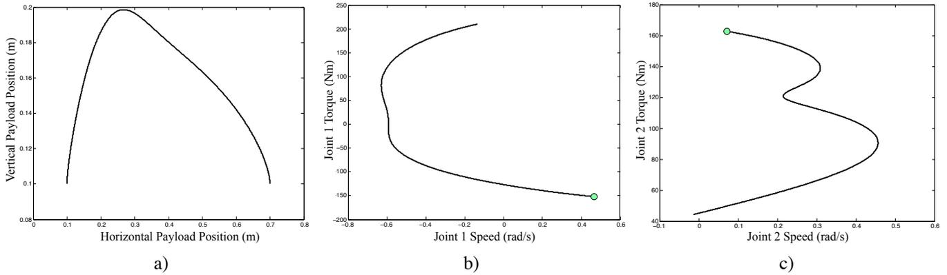
Figure 2: Optimal trajectories for nominal plant design: a) Payload trajectory b) Joint 1 and c) Joint 2 torque-speed trajectories.
