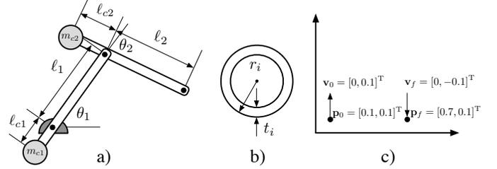
Figure 1: a) Counterbalanced two-link planar manipulator. b) Section view of link  $i$ . c) Task A initial and final conditions.
