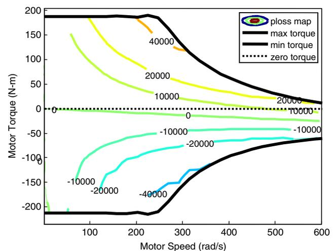
**Fig. 8** Optimal motor map, ATC-POD
