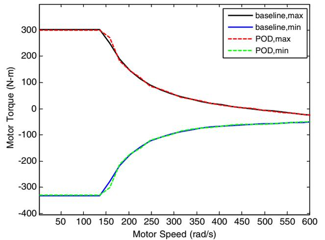
**Fig. 11** Torque curve comparison, POD approximation and baseline
