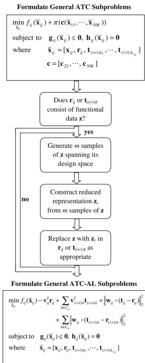
Fig. 2 Flowchart for reduced representation in ATC
