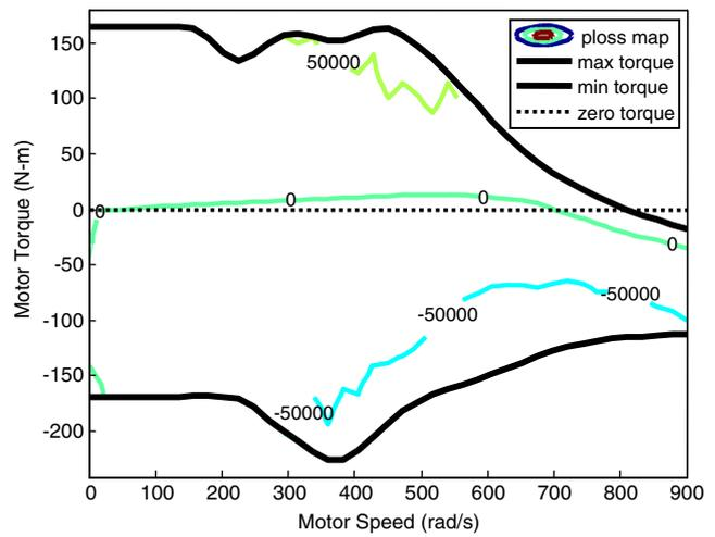
**Fig. 6** POD-approximated motor map at failed design point
